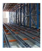
**Pallet Flow** Uses gravity and wheels or rollers, to convey and accumulate pallets in a storage module. Depths can range from 2 to over 20 pallets deep, thereby giving vou higher storage density than other forms of racking.
