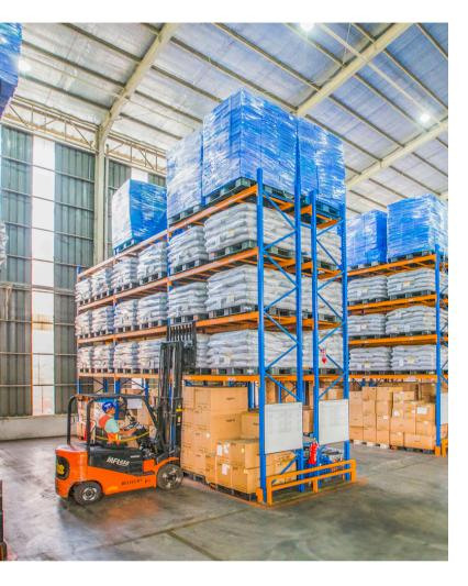
Pallet racking is the backbone of modern warehouse storage systems, providing a structured and efficient way to store goods. It consists of upright frames, horizontal beams, and wire decking or wooden pallets to support inventory.
