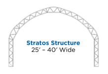
Offers maximum height clearance and interior space with a minimal footprint. Featuring a straight, extra-tall leg frame and multiple side entry options, it simplifies storage for large equipment and commodities. The engineered truss frame makes it ideal for townships and municipalities seeking efficient storage within city limits.
