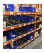
The rack supports inclined rollers or wheels that allow cartons to glide from the back (loading) aisle to the front (picking) aisle. When the front carton is unloaded, the next automatically glides into picking position for increased picking efficiency.
