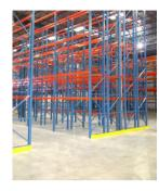
**Double Deep** A double deep racking layout involves back to back rows of 2 deep selective rack. Each pick slot now has a front and a back pallet.
