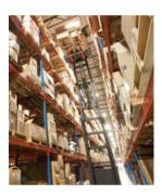
**Very Narrow Aisle** Maximizes warehouse space by reducing aisle width, allowing for efficient access to goods using specialized narrow aisle forklifts.
