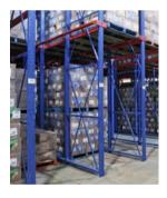
**Drive-In** Allows standard fork truck access into the face of the system allowing larger storage blocks which reduces the number of required aisles.
